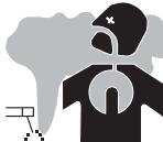
The fumes, gas and dust generated by cutting are a potential health hazard. It is mandatory to ensure adequate ventilation and/or extraction to keep fumes and gas away from the work area. Using an air fed welding helmet is recommended in case of insufficient ventilation in the workplace.
