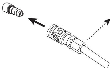
Connect the gas supply to the power source using an inert gas pipe with an internal diameter of 9.5 mm and a quick release connector.
